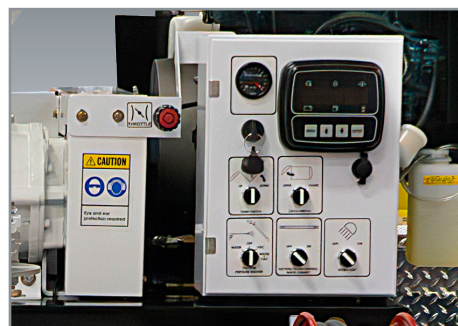
All major systems and operating controls are located curbside for operator safety
